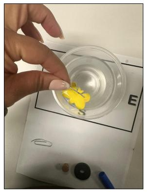
5. It will start to spin slightly so the magnetized end will point north. If it starts to bump into the edge of your cup or bowl, gently push it to the centre and let it realign itself until it consistently points in the same direction.
